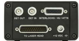
Laser controller CT. Rear view
