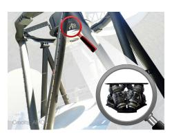
The hexapod is installed on Pan-STARRS-2 telescope at an altitude of 4267 m on Maui, Hawaii. A smaller version of SURES has been adapted as the secondary mirror is 600 mm diameter and weighs less than 110 kg.
