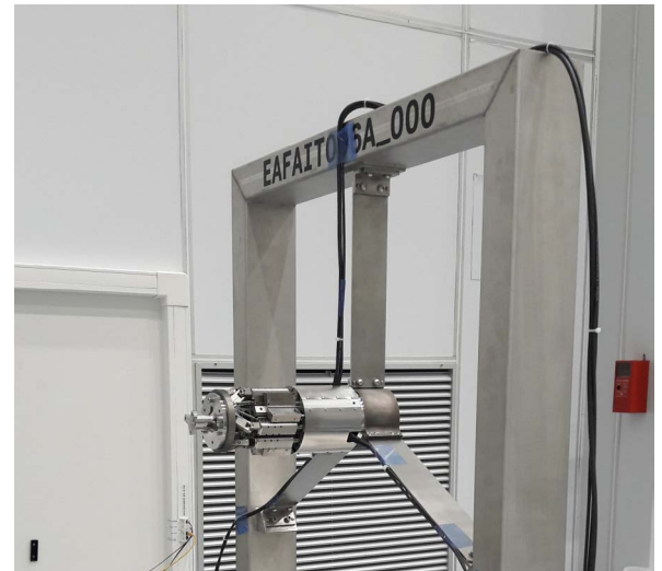
MAUKA hexapod has a very small diameter of 107 mm.
