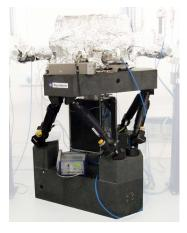
JORAN hexapod has been developed in collaboration with ESRF synchrotron to position mirrors with very high resolution.
