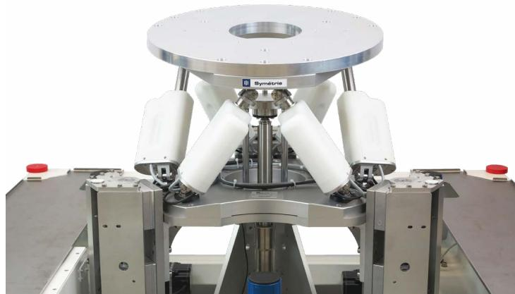
This BREVA hexapod is coupled to a Tz stage in order to achieve  $\pm 6^\circ$  rotation at a pivot point 1400 mm away from the hexapod. It is used to calibrate a space optical instrument developed by Leonardo.
